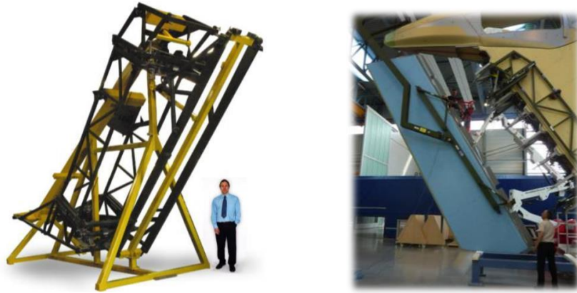
A400M Tooling Support –Rudder Removal & Installation Tool
