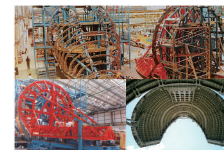
Beluga Door, Tooling Design, Manufacture & Installation into 1st Aircraft.
